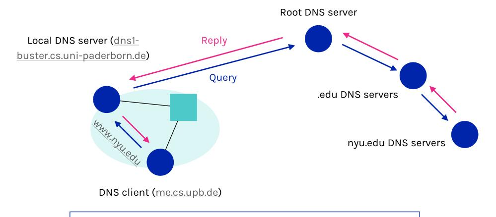
The client offloads the task of resolving to the server recursively
