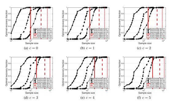
Figure 4: Sample complexity for finding the approximately most probable ranking (AMPR) with parameters  $M \in \{5, 10, 15\}$ ,  $\delta = 0.1$ ,  $\epsilon = 0$ . The results are averaged over 100 repetitions.
